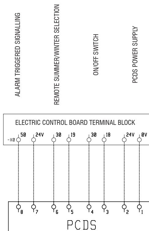
Note: Should the unit go into an alarm status, a voltage of 24V will be present on the terminals of the electric control panel; where an interface with a voltage-free contact is desired, a relay must be fitted by the installer.
